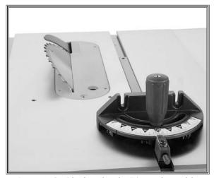
Figure 48. Blade tilted 45° to the table.
